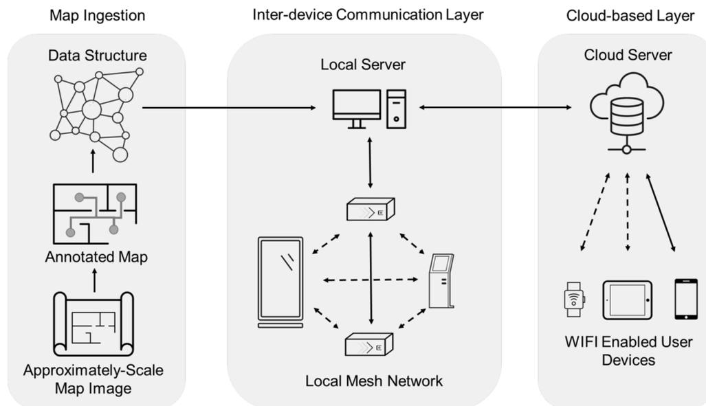
Fig. 4. A diagram showing three layers of the system including map ingestion, inter-device communication, and cloud-based servers. The diagram uses icons of mobile devices, different display units, computers, and data structures to provide an overview of the current and future system using solid and dashed lines.
