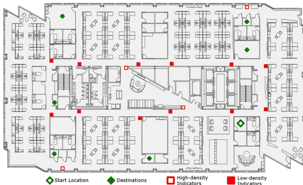
Fig. 9. The actual floor plan of the evaluation site showing long hallways, numerous offices, cubicle areas and a meeting space on a diagonal in the center. Highlighted on the map is all the indicators and destination locations.
