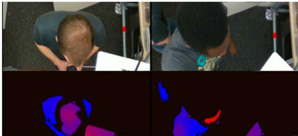
**Figure 7.** Color (top) and depth (bottom) image of two human subjects with different hair types as measured by an active infrared stereo camera. The depth map is color-coded such that darker (more black) is farther away from the camera while lighter (more red) is closer.
